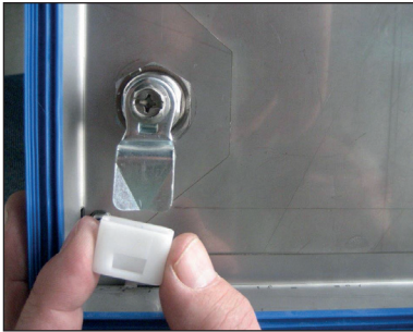
Slide on latch shoe
